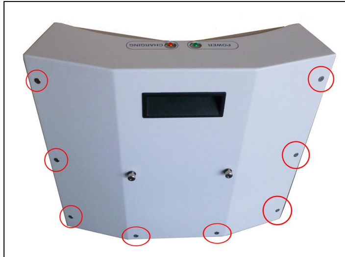
Figure 8-16 Docking Station Rear Cover Screws (8 of 10)
